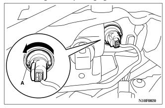
Turn the light socket (A) counterclockwise and pull it out and remove the light bulb.
